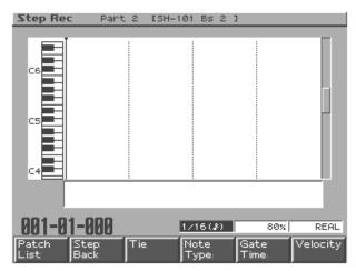
Use function buttons [F4]–[F6], and [VALUE] and [INC/DEC] to specify the length and velocity of the notes to input.
